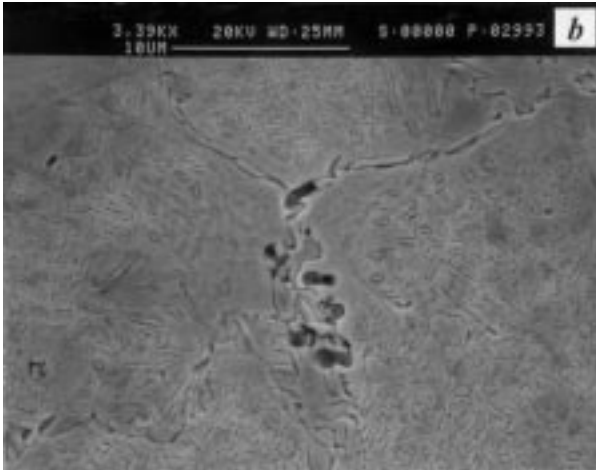
Figure 6 (a,b) (SEM-SE) Alloy A simulating veneering treatments before (a) and after electrochemical test plus light metallographic etching (b).
